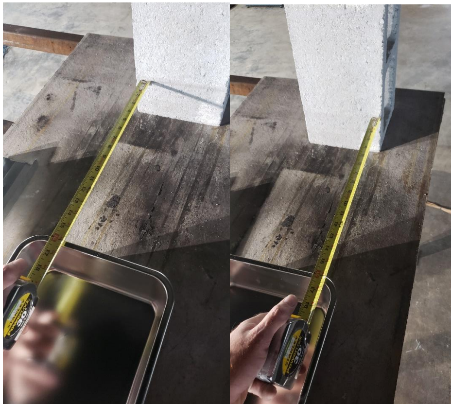
Photograph No. 4: Test pan spacing from brick as measured from both sides of pan to ensure squareness (typical for all tests).
