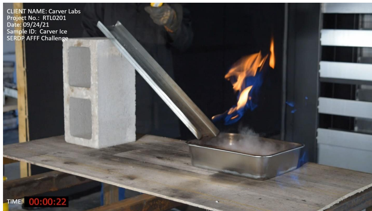
Photograph No. 14: Typical flame immediately prior to flame fully extinguished.
