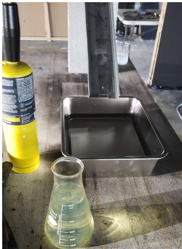
Photograph No. 6: Test setup prior to pouring gasoline into test pan (typical for all tests).
