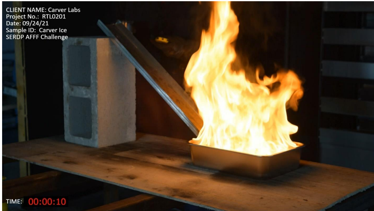
Photograph No. 10: Test Flame after pre-burn period of at least 10-seconds (typical for all tests).
