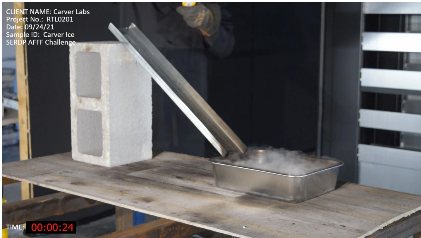
Photograph No. 15: Typical flame immediately after flame fully extinguished.
