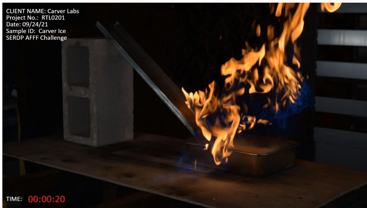
Photograph No. 13: Test Number 2 five seconds after pouring of carver Ice down ramp.
