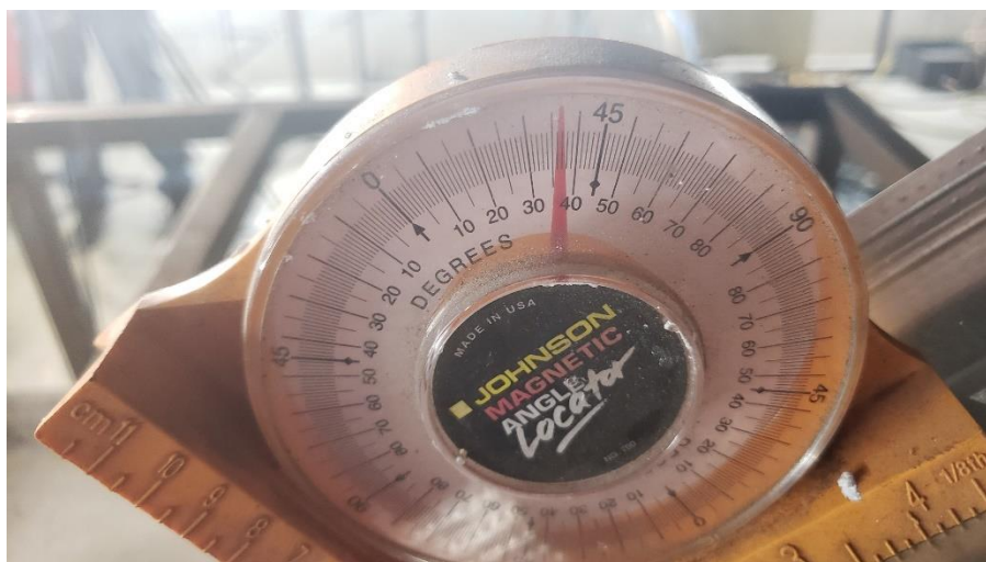
Photograph No. 3: Metal Track Ramp angle of 36.5° after installation onto test pan and block.
