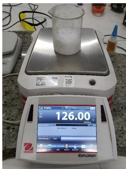
Photograph No. 7: Beaker being weighed immediately prior to igniting the test pan (typical for all tests).
