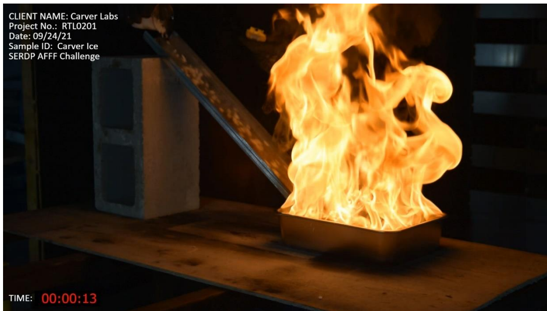
Photograph No. 11: Start of pouring fire extinguishing component Carver Ice pellets down ramp (typical for all tests).
